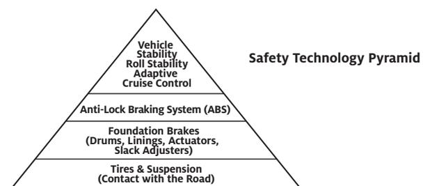
This is illustrated in the “Safety Technology Pyramid” shown below. Vehicle braking and stability is first determined by the tires and suspension, which determine the how much of the tire is proper contact with the road, followed by proper foundation brake operation and so on. The technologies further up the pyramid are dependent on the technologies below them to be properly operating in order for the more advanced technologies to be fully effective.
