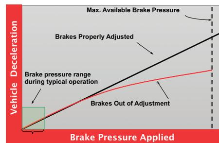
Relationship Between Brake Adjustment and Vehicle Deceleration
